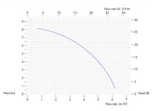
The curves and performance values refer to pumps with free delivery outlet with water at 20 °C, and two poles motor 50 Hz These data may vary according to the construction materials and hydraulic conditions.
