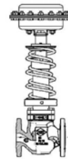
Alternative mounting position for gases and liquids at medium temperature up to 80 °C. Not for steam.
